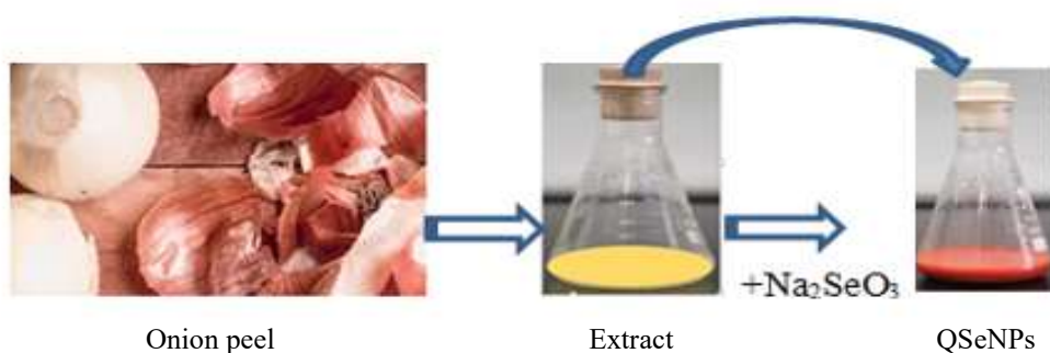
Fig.1. Synthesis of nanobioconjugates of selenium and quercetin using aqueous onion peel extract.
