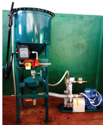
Fig. 1. The circulation mixer-separator for vegetable oil transesterification
