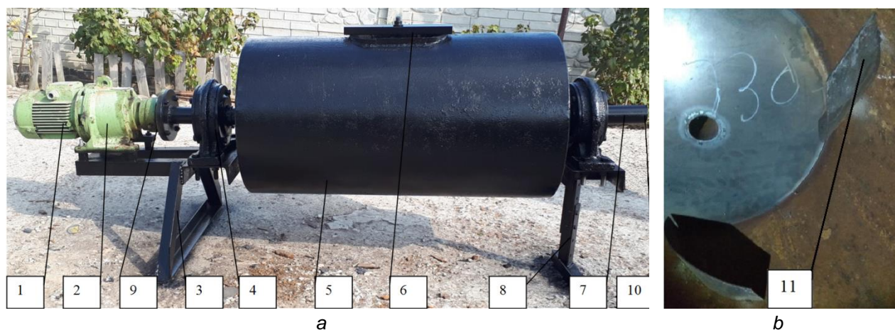
Fig. 1 – Experimental installation: a – general view of a drum type reactor; b – blades installation
